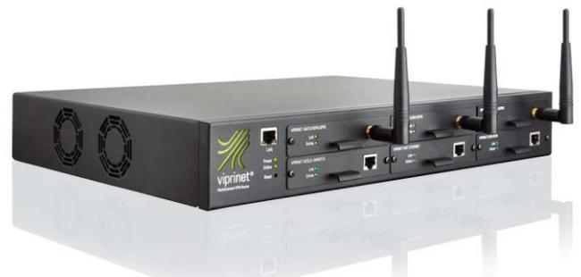
This 19"-sized router allows the bonding of up to six different WAN lines into a single, high-performance virtual link. Whether it is used for site link even in remote areas at home or abroad, for integrating home offices or road warriors into the company VPN, or for establishing a reliable and fast Internet link in rural areas: The Multichannel VPN Router 1610 offers ideal bonding capacities for setting up company networks of different sizes. The router is particularly robust and persistent.
